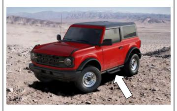
1. If fitted, remove the factory side steps.
