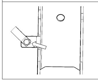
13. Using P-Clip provided, attach the wiring harness with an M6x25 bolt and washer to the rear mount cage nut, so that the harness will not rub.
