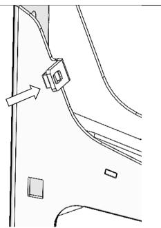
8. Insert M6 cage nut into rear mount of left slider.
