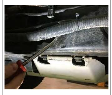
6. Using a clip removal tool, loosen the wiring harness from the length of the left side frame rail. On the inboard side of the left frame rail, also disconnect the brake lines in the rear.
